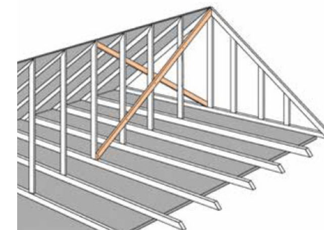
Figure 4-14. Diagonal bracing runs from the top of the gable end to the bottom of the fourth truss, and from the top of the fourth truss to the bottom of the gable end. (Source: FEMA’s “Against the Wind” brochure)
