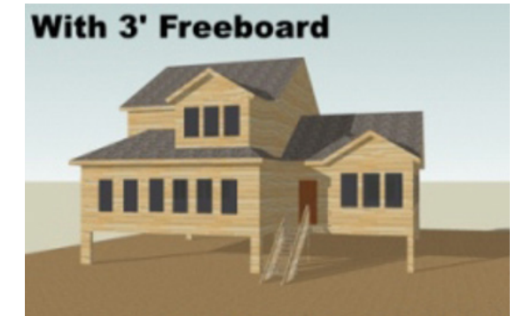
Figure 4-33. House on the right elevated with freeboard. (Source: FEMA)
