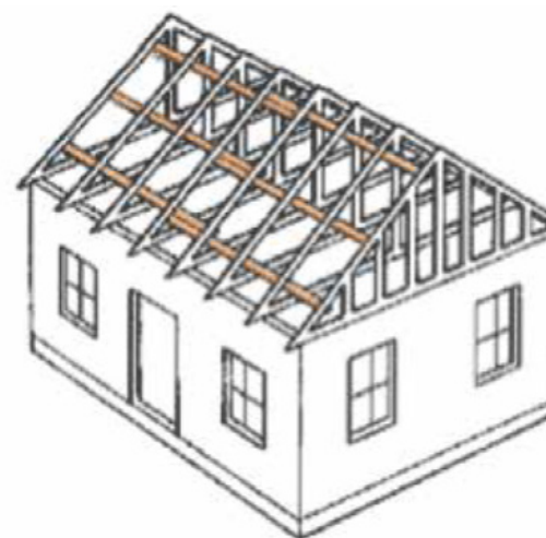
Figure 4-13. Lateral bracing consists of 2x4s running the length of the roof and overlapping where they meet each other. (Source: FEMA’s “Against the Wind” brochure)
